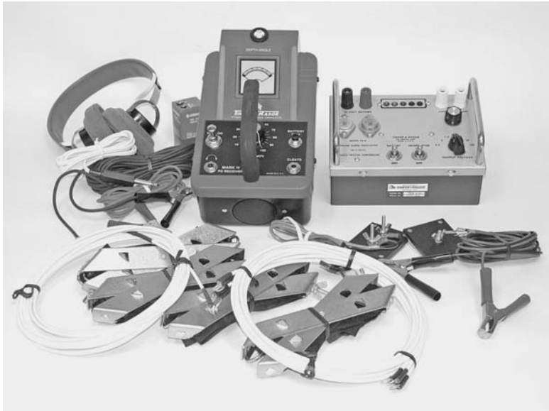
FIGURE 13.37 Instrumentation to carry out a Pearson survey. (Photo courtesy of Tinker & Rasor)
