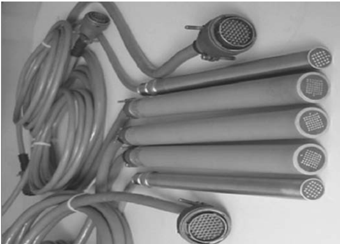
FIGURE 5.39 Typical CMAS probes used for real-time corrosion monitoring. (Courtesy of Corr Instruments, LLC)
