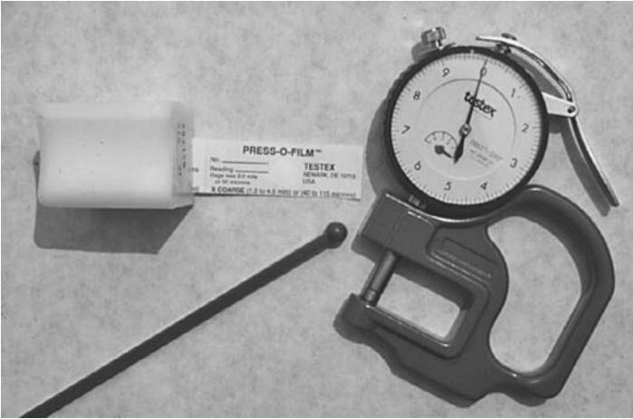
FIGURE 14.22 Testex Press-O-Film replica tape surface profile measurement equipment. (Courtesy of KTA-Tator, Inc.)
