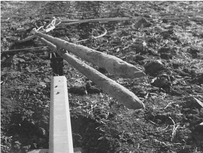
FIGURE 7.15 Anchor assembly cut by corrosion at the concrete anchorage. (Courtesy of Anchor Guard)
