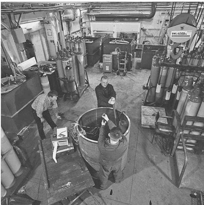
FIGURE 11.29 Full-ring test in preparation for a 45-in pipe. (Courtesy of CAPCIS Ltd.)
