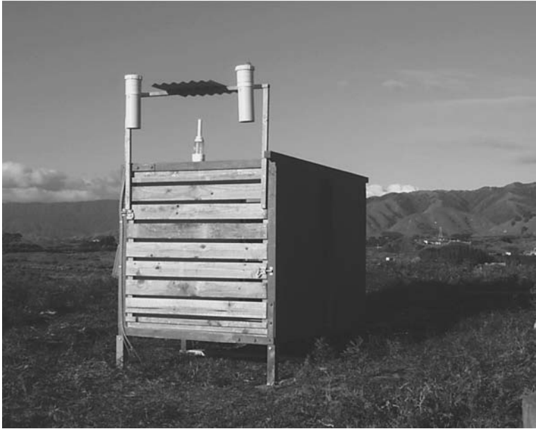
FIGURE 9.25 Subfloor simulation box surmounted by a wet candle chloride measuring device that has been installed at several sites in Australia and New Zealand. (Courtesy of Branz, New Zealand)
