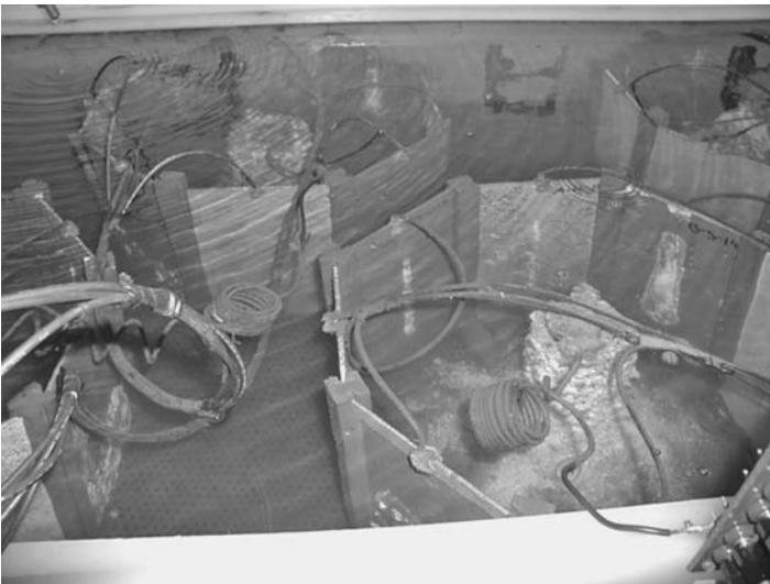
FIGURE 14.30 Laboratory setup to test for disbonding during the application of cathodic protection. (Courtesy of Corpro)
