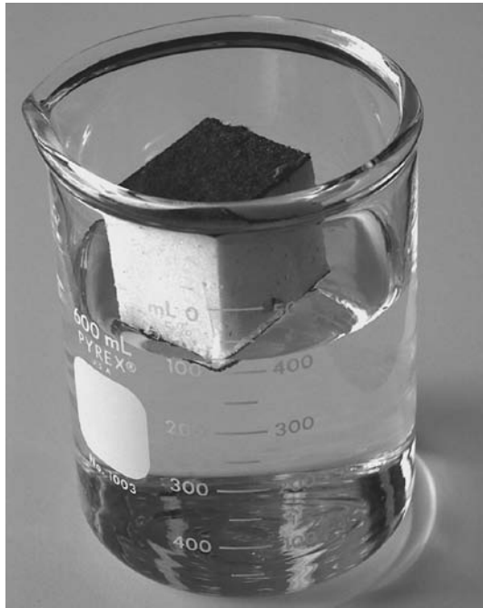
FIGURE 6.27 Sample of isocyanurate foam still floating on water after six weeks.
