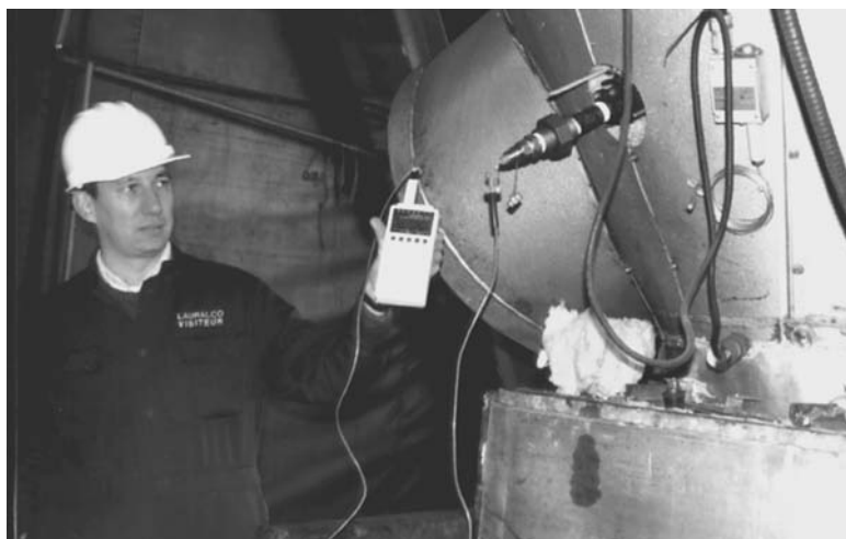
FIGURE 5.34 Field corrosion monitoring using electrochemical noise recorded with a handheld data logger. (Courtesy of Kingston Technical Software)
