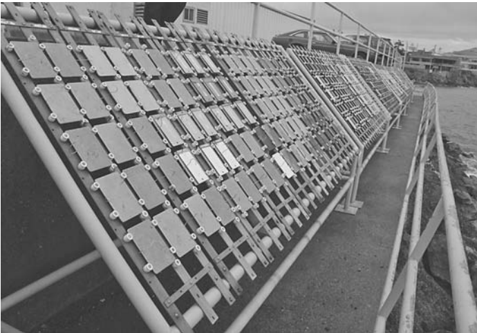
FIGURE 9.39 Atmospheric test rack exposed to marine West Coast environments. (Courtesy Defence R&D Canada-Atlantic)
