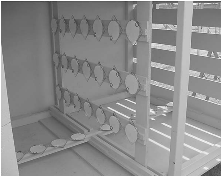
FIGURE 9.26 Horizontal and vertical filter papers installed inside a subfloor simulation box. (Courtesy of Branz, New Zealand)
