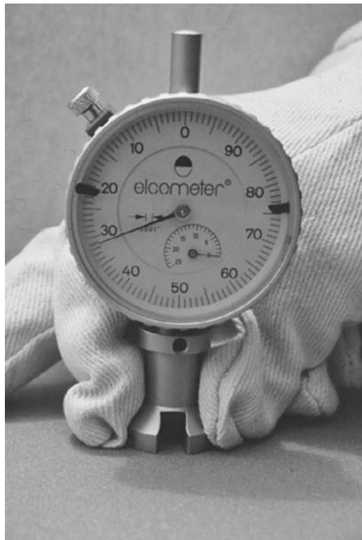
FIGURE 14.21 Measuring surface profile depth using depth micrometer. (Courtesy of KTA-Tator, Inc.)
