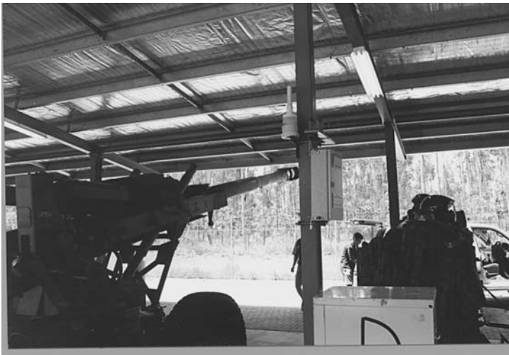
FIGURE 9.42 Semisheltered test station with test coupons, wet candle apparatus, and data logger attached at an army base in Northern Australia. (Courtesy of DSTO Australia)
