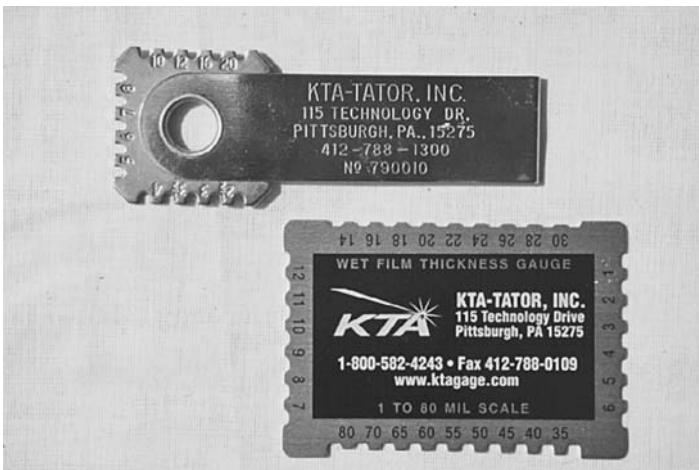
FIGURE 14.25 Notch-type wet film thickness gauges (top: stainless steel; bottom: aluminum). (Courtesy of KTA-Tator, Inc.)
