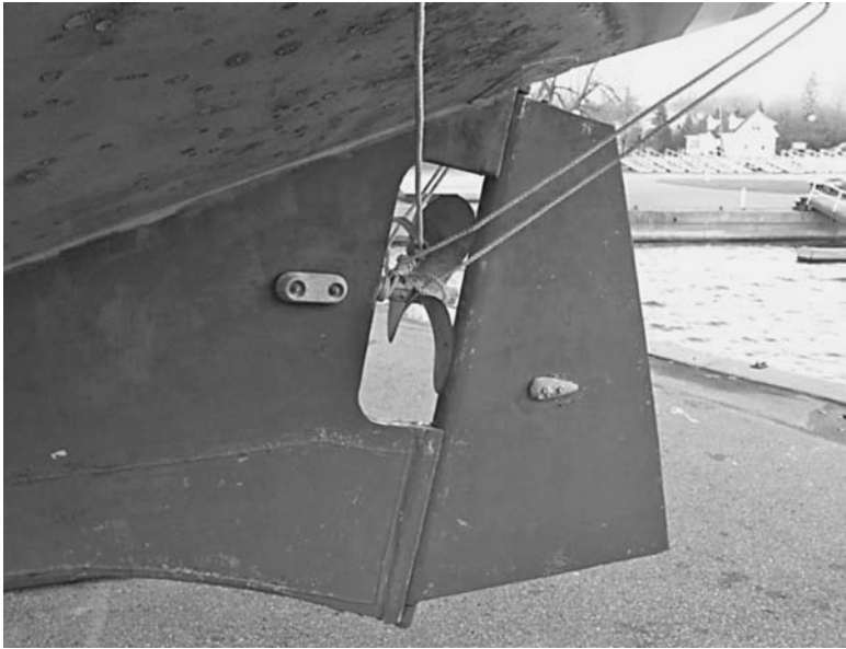
FIGURE 13.4 Sacrificial zinc anodes on a sailboat. (Courtesy of Kingston Technical Software)
