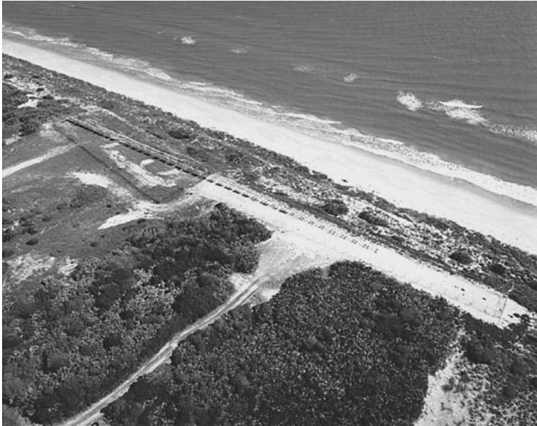
FIGURE 9.27 Aerial view of the NASA Kennedy Space Center beach corrosion test site where atmospheric corrosivity is the highest corrosivity of any test site in the continental United States.
