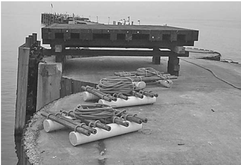
FIGURE 13.26 Sleds with six cast iron anodes, integrated cable, and protective hose for an operation capacity of 75 amperes for fifteen years. (Courtesy of Dean Rookes, West Coast Corrosion Prevention Ltd.)
