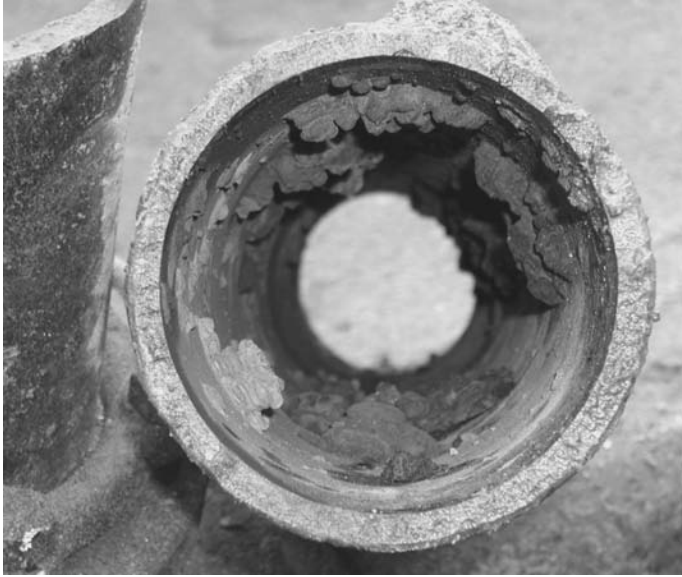
FIGURE 6.10 Corrosion products forming nodules or tubercles over pit cavities. (Courtesy of Drinking Water Services, City of Ottawa)
